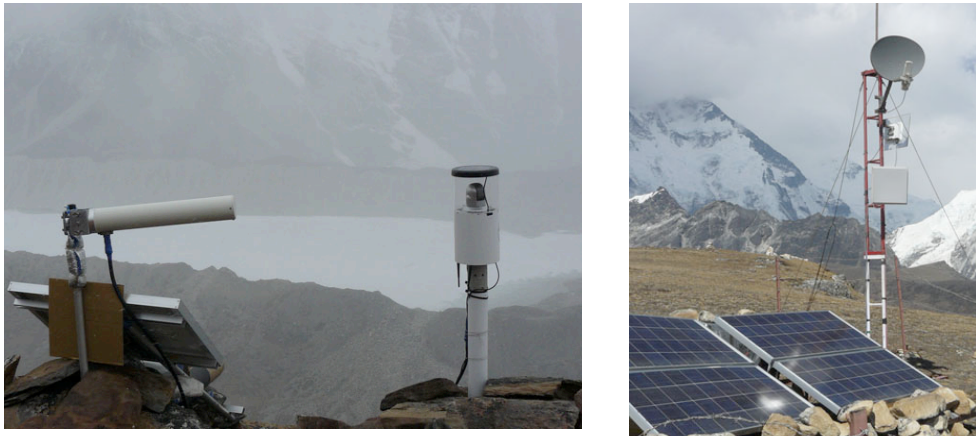
Figure 7. field servers and wireless relay station for monitoring Imja Lake (5000m)
