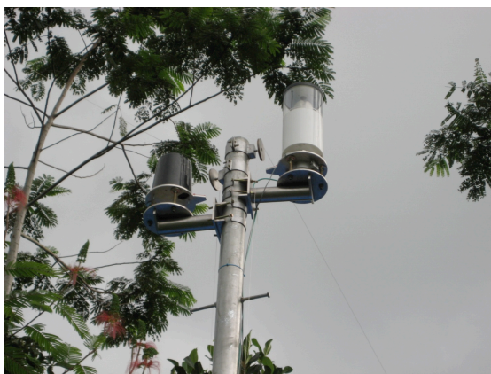
Figure 6. The fixed pole with rain gauge and network camera, and the outdoor box with fieldserver and other associated circuits
